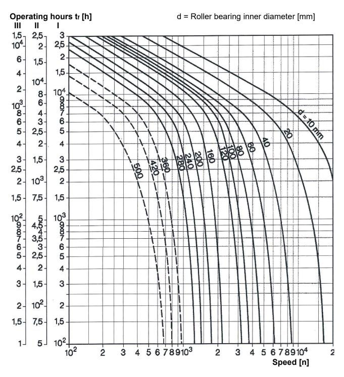
**Scale I:** Radial ball bearings; **Scale II:** Cylinder roller bearings; **Scale III:** Spherical roller bearings
