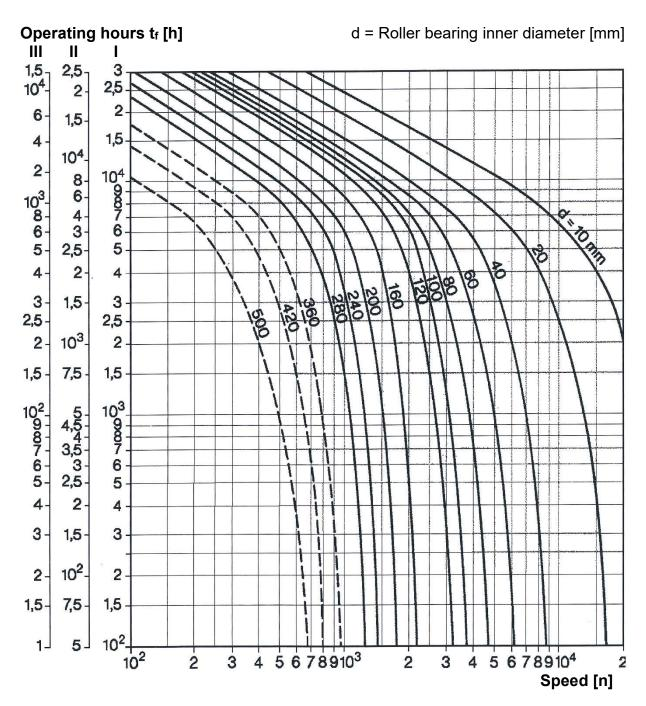
Scale I: Radial ball bearings; Scale II: Cylinder roller bearings; Scale III: Spherical roller bearings Reduce the determined lubrication interval tf [h] by 50% for:
